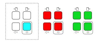
Page Buttons Navigate up and down through pages with utility buttons. When in auxiliary mode the shift button will illuminate coloured cyan.
